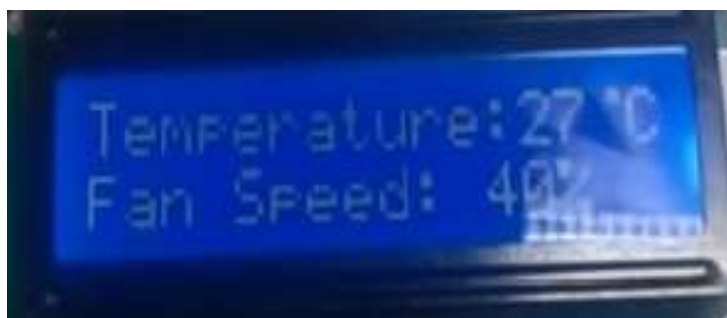
Fig. 11: LCD displaying temperature and fan speed
