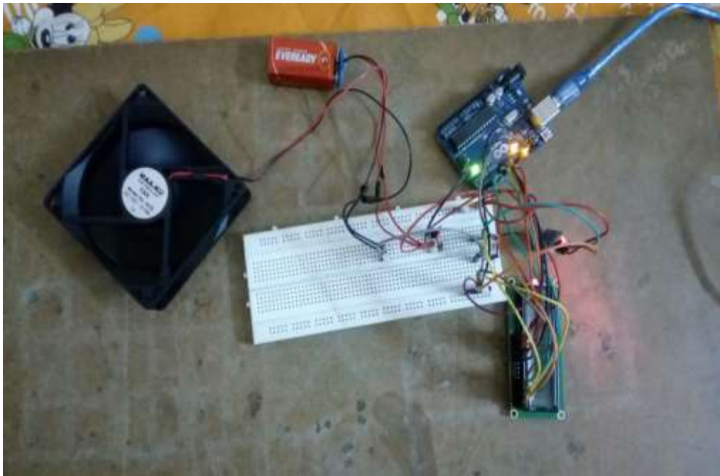
Fig. 9: Connections of controlling rotation of the fan in accordance with the temperature of the cabin
