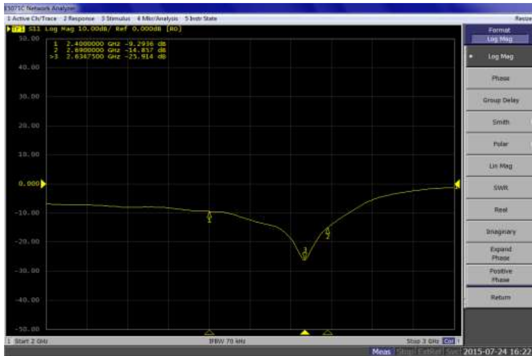
Fig. 15: Measured return loss vs. frequency curve on VNA
