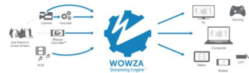
Fig. 27. Wowza Streaming Engine accepts video from a variety of sources and outputs to multiple formats
