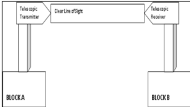
Figure 3. Block Diagram of Working Principle of FSO system.
