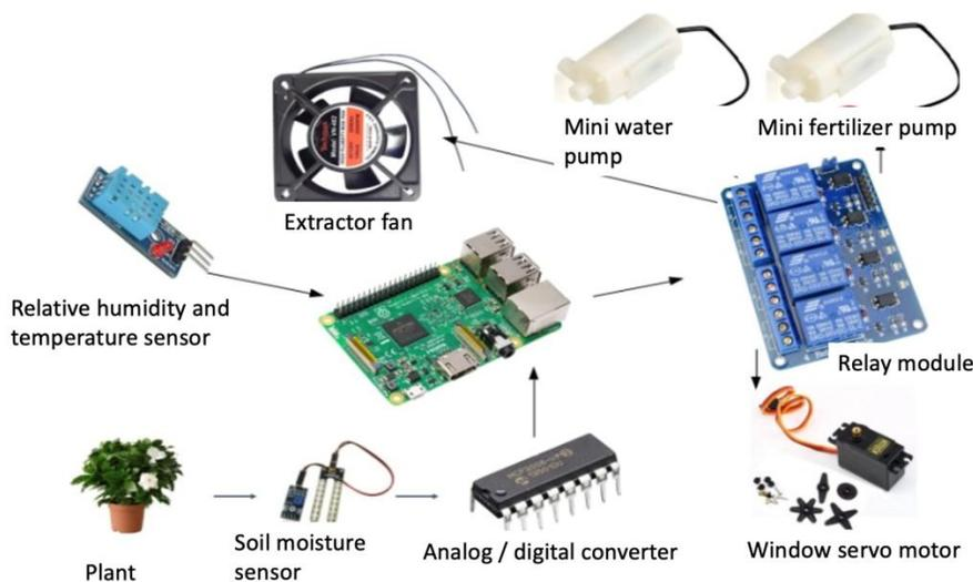
Figure 2. Sensor and actuator connection diagram.
