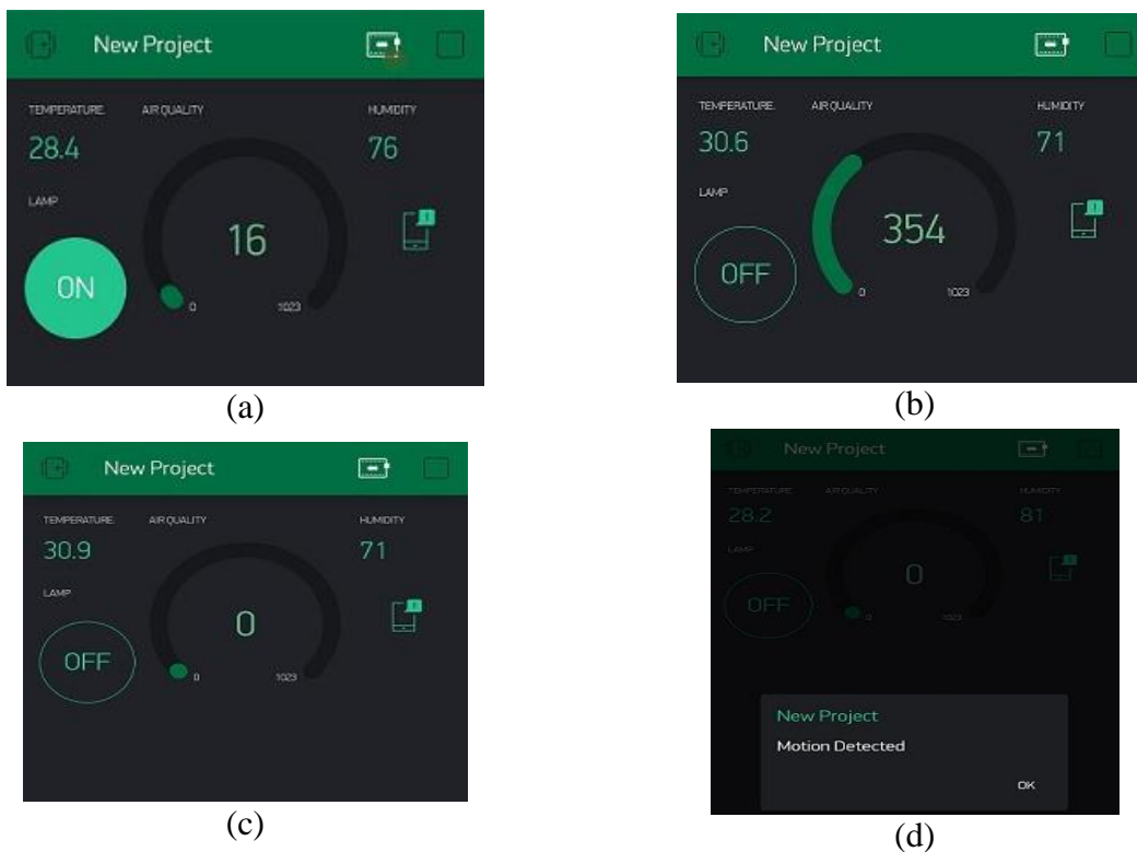
Figure 4 Blynk app interface, (a) ON Lamp / humidity test, (b) Air Quality/temperature test, (c) Air quality test, (d) Motion detector test
