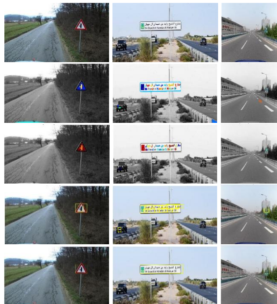
Figure 5 (Top to bottom) 1st-6th rows: input image, MSER regions, after eliminating non-text areas based on geometric properties and thinning operation, expanded the text of bounding boxes and final result
