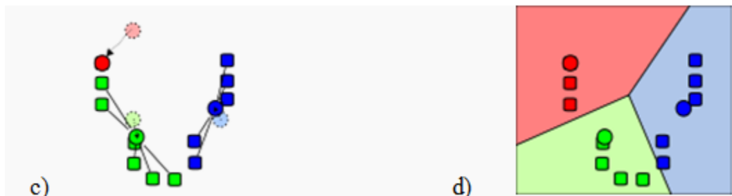
Figure 2.3 (c,d) Demonstration of the Standard K-means Algorithm (Wikipedia, 2016).
