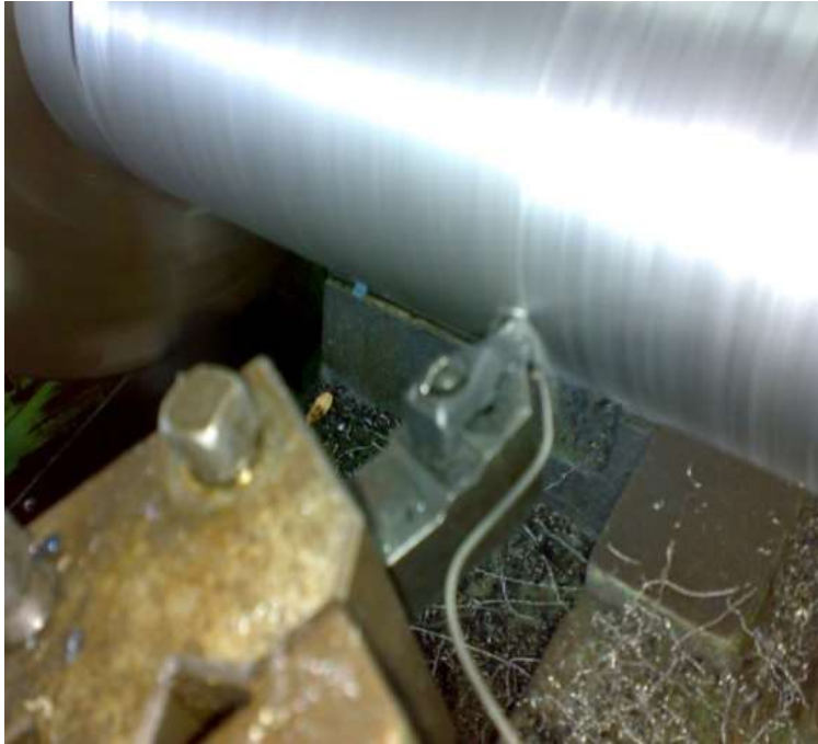
Fig. 3 Actual tool temperature measurement showing thermocouple wire and holder
