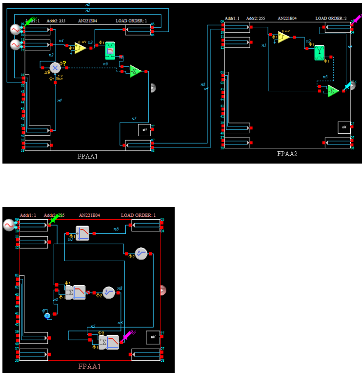
Figure 7. Linearization of a magnetic field sensor.
