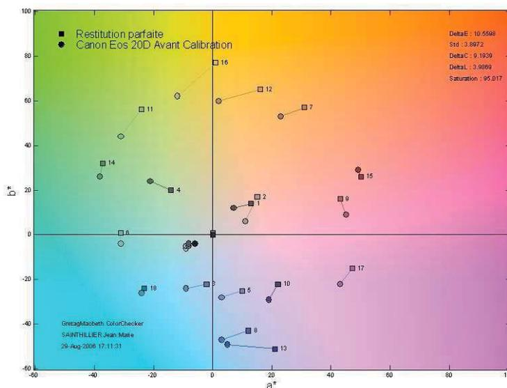
**Figure 7 Example of colorimetric characterization of a Canon Eos 20D**
