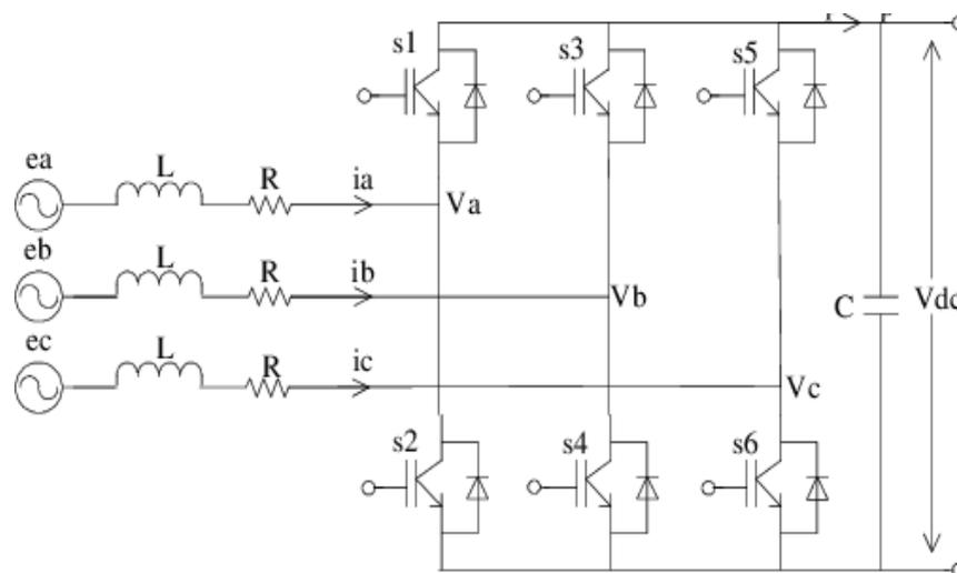
**Figure 1 Circuit diagram of static synchronous compensator**
