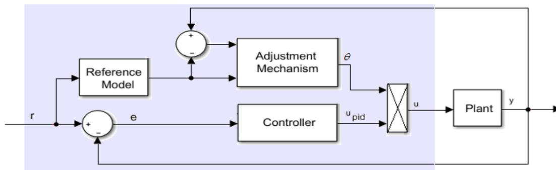
**Figure 4(a) Block diagram of Model reference adapted controller**
