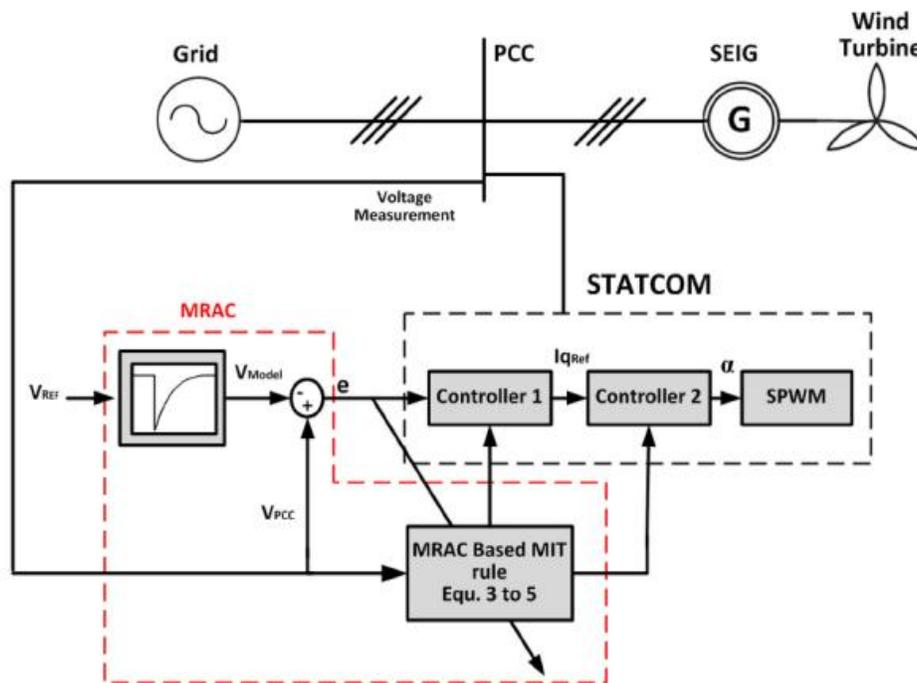
Figure 4(b) Block diagram of Model reference adapted controller integrated to grid
