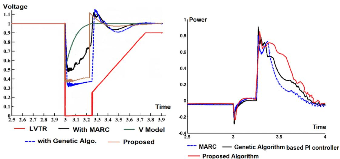
Figure 6a) Comparison of voltage at PCC Figure 6b) PI- GA and MRAC reactive power comparison
