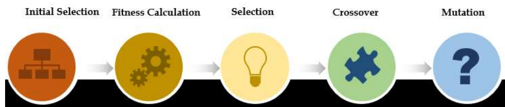
Figure 1 Operational Flow of Genetic Algorithm
